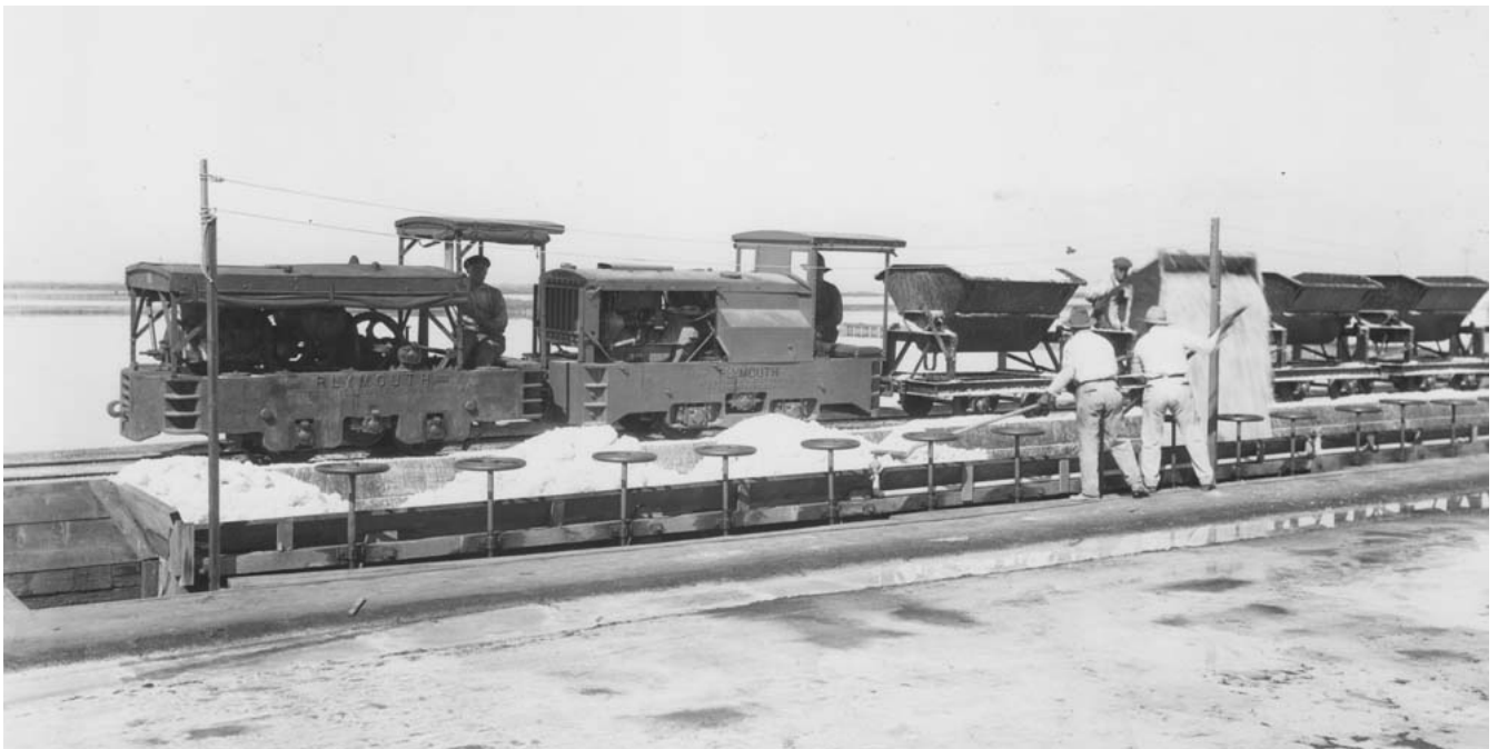
The two Plymouth Gasoline Locomotives owned and operated by the Western Salt Company. ( The San Diego Union , July 1, 1924.)
