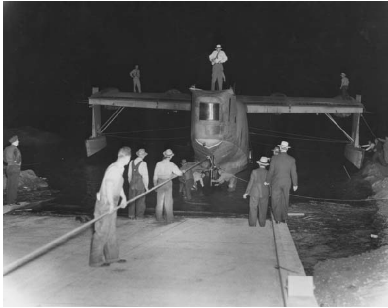
A Consolidated PB2Y3 is hauled up the seaplane ramp at Rohr for conversion to carry cargo in June 1943.
